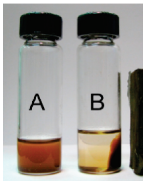
Figure 6. Photographs of (A) \gamma -Fe 2 O 3 nanoparticles stabilized by 1:1 block copolymer NC1-B2 in cyclohexanone and (B) the same ferrofluid under the influence of external magnetic field.
